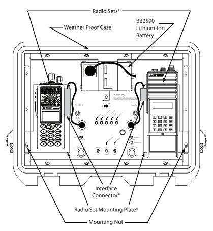
\*Interface connectors and mounting plates are dependant radio set type. Contact BK Technologies for available radio types.
