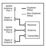
To disconnect the duplexer and use the two antenna ports, perform the following steps:
