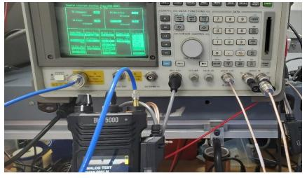
j. On HP8920, in RX Test mode, place the cursor to AF ANL under To Screen box then press the cursor control knob. It should go to the next screen.
